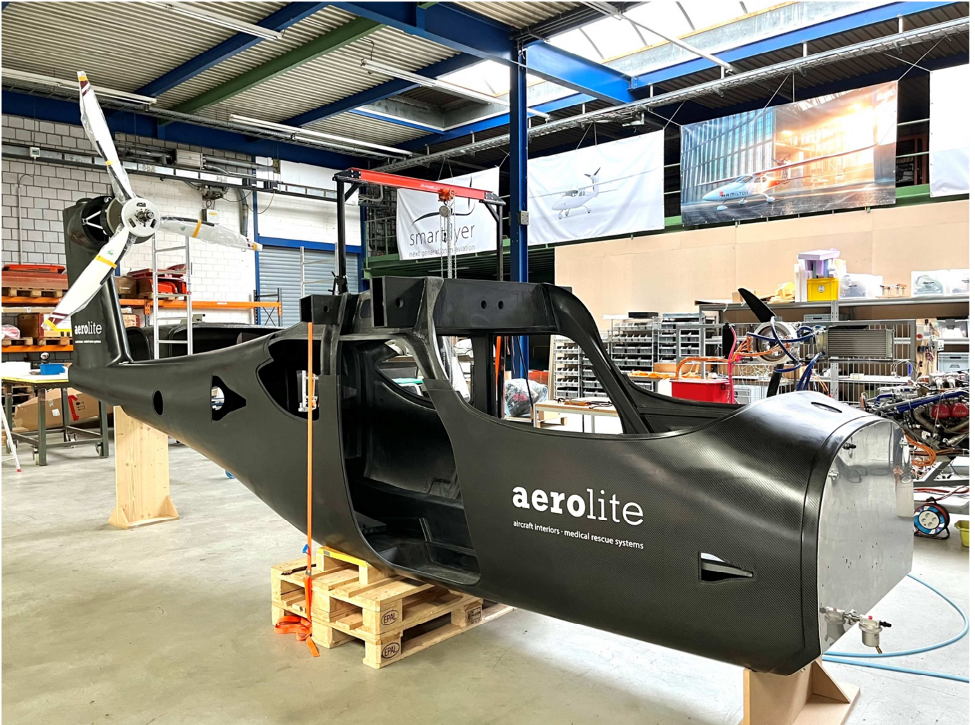
Carbon fibre fuselage of the smartflyer with drive unit in the vertical stabilizer
